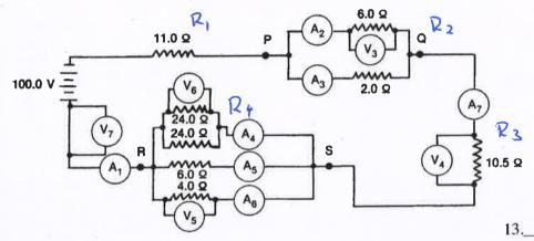
14. Calculate the reading for each of the 7 ammeters in the circuit diagram below
