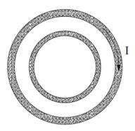
An increasing current flows clockwise around the outer ring.
