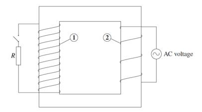
Which of the following correctly identifies Part 1 and Part 2 and the function of this transformer?
